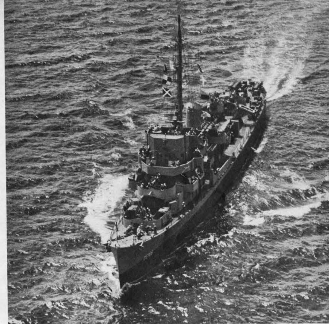
Head-on views contrast lightly shielded superfiring guns on U.S. DE's foredeck (above) with DE UN-1's large single gunhouse (below). U.S. main armament is three in., Japanese, 4.7 in. U.S. DE shown is of Evarts Class, shorter but essentially similar to Buckley Class.
